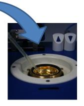
Measure of the induction time thanks to the RSSOT - **Rapid Small Scale Oxidation Test-** performed at high temperature and under oxygen pressure. Possible application for oils, fatty phases and finished products.
